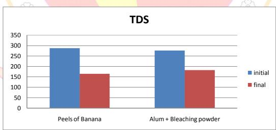
Initially, we recorded turbidity 8.7 NTU in sample 1 which is get minimized after treatment of peels of banana up to 4.2 NTU and 3.9 after treatment of Alum + bleaching powder. In case of Total dissolved solid, initially it is recorded 287 mg/L and finally we observed 164 mg/L in case of banana peels treatment.
